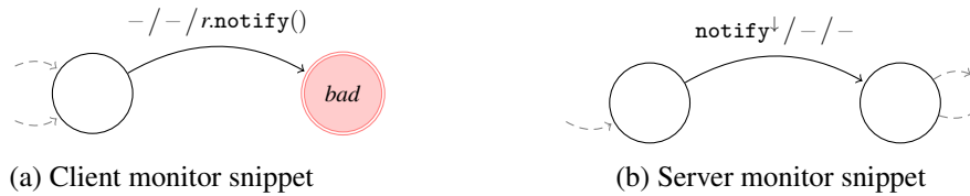
Figure 6: Synchronisation of monitors using active objects. Here r is an active object with a public method notify() , that is instantiated by the server monitor and called by the client monitor (for notifying the server monitor).
