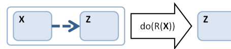
FIGURE 5 – Modification of the graph of a Bayesian network after a probabilistic intervention on a subset of variables. The bold dotted arrow represents the set of arrows from any node of the set \mathbf{X} to any node of the set \mathbf{Z} .
