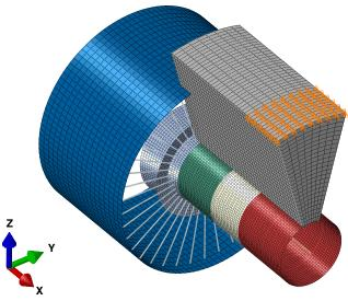
Fig. 1 Engine and design zone (in gray) finite element model. The engine model is made of 9976 finite elements, 9312 linear quadrilateral elements with reduced integration, and 664 linear beam elements. The solid design zone is clamped at the orange points.
