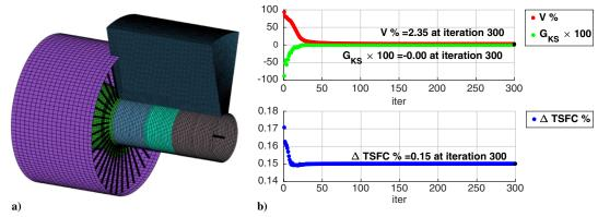
Fig. 7 a) Design zone mesh used for final topology optimization problem. Each element of the original element is cut into 64 new elements, which give a total of  $7600 \times 64 = 486,400$  eight-node linear 3D solid finite elements and 509,949 nodes. b) Convergence history of  $\Delta TSFC \%$ , V %,  $G_{KS}^l \times 100$  after 300 design iterations.
