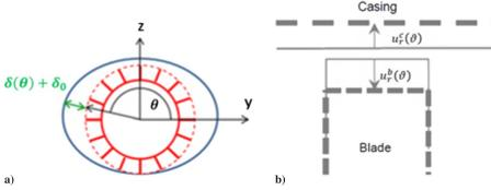
Fig. 2 Rotor and stator displacements under maneuvers loads: a) z-y engine section diagram for a given rotor stage. The red structure stands for the rotor; the blue line for the deformed stator. b) Diagram illustrating radial displacement effect on the total tip clearance. The resulting tip clearance is the sum of the initial clearance  $\delta_0$  and its variation induced by the engine deformation calculated as  $\delta(\theta) = u_r^c(\theta) - u_r^b(\theta)$ .
