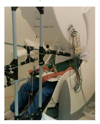
**Fig. 1.** The experimental setup for brushing on the lower arm. A curtain blocked the participants' vision of the brush movement. A fiber-optic sensor, that marked the timing of the contact between brush and skin, was attached alongside the bristles of the brush.
