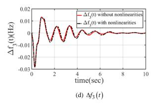
Figure 13. Response with nonlinearities under step load disturbance
