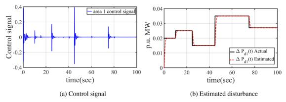
Figure 12. Response using proposed design under random step load disturbance
