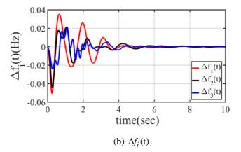
**Figure 15.** Response with IEEE 39 bus system under step load disturbance
