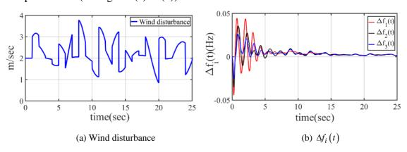
**Figure 14.** Response with an integration of wind energy under step load disturbance
