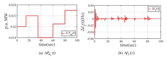
**Figure 10.** Response using proposed design under random step load disturbance
