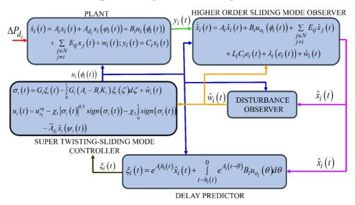
Figure 2. Block diagram of prediction-based ST-SMC using DO
