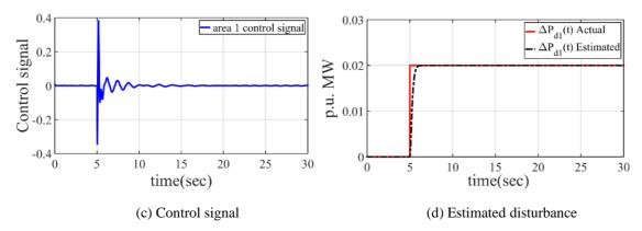
**Figure 5.** Response using proposed design under step load disturbance
