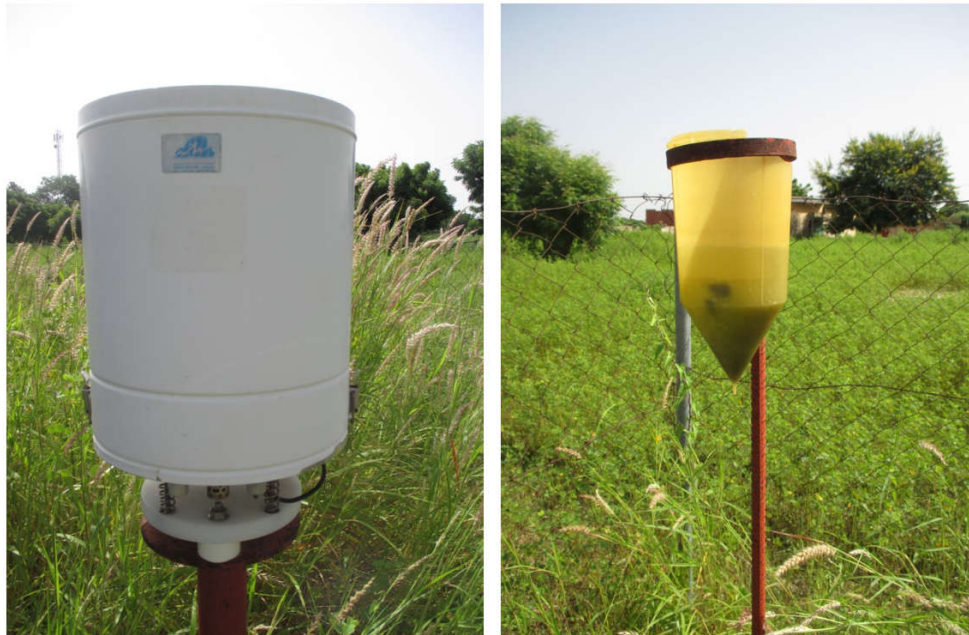
Figures 1 and 2: An automatic (left) and a handcrafted rain gauge (right), in the village of N'Doffane. (Pictures taken by the author on 5 October 2017.)
