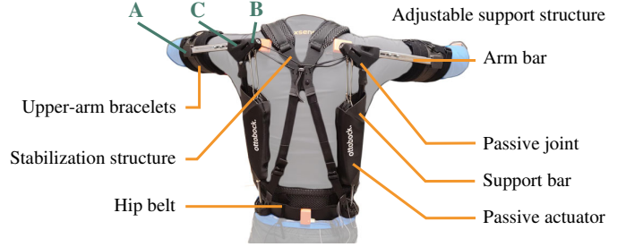
Fig. 1: PAEXO consists of a stabilization structure attached to the participant and a support structure transferring a portion of the arm weight from the upper-arm bracelets to the hip belt.
