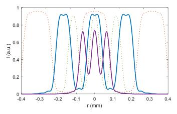
**Fig. 4.** Simulated 1D raw image with the three effects versus position r on the detector for different depths  $z_0$ :  $z_0^{\text{ref}} = 233 \text{mm} \ (blue)$ , 231mm  $(dotted \ orange)$ , 235mm  $(dotted \ green)$ , and 240mm (purple, same depth as in Fig. 3).
