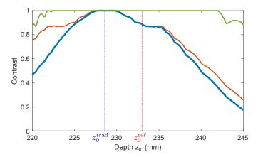
**Fig. 5.** Contrast curves versus depth: with defocus and magnification only (*green*), with diffraction and magnification only (*orange*) and with the three effects combined (*blue*). Depths  $z_0^{\rm ref} = 233 \, \rm mm$  and  $z_0^{\rm trad} = 228.6 \, \rm mm$ . Note that the small oscillations are due to pixel discretization of the signal.
