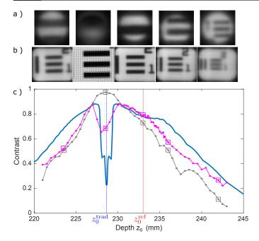
**Fig. 6.** a) Raw sub-images acquired at planes:  $z_0 = 223.5$ , 228.5, 233, 236, 242mm; b) Corresponding reconstructed images; c) Comparison of the simulated contrast curve (*blue*) and experimental contrast curve measured on raw sub-images (*pink*) and on reconstructed images (*gray*). The gap located around  $z_0^{\rm trad} = 228.6$ mm is due to the large magnification that makes the bars exceeding the sub-image size.
