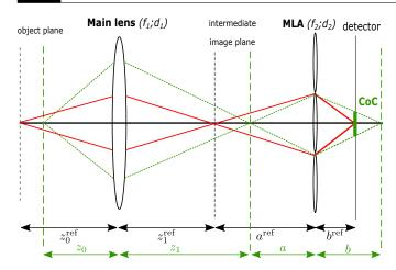
**Fig. 1.** A focused plenoptic system. Red rays come from the reference depth plane  $z_0^{\text{ref}}$  whereas green rays correspond to another depth to illustrate the Circle of Confusion (CoC) due to defocus.
