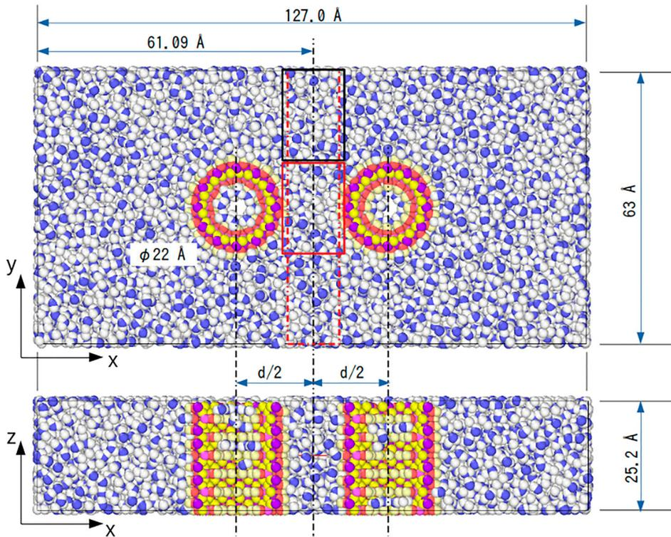
**Figure 2.** Simulation setup: plan (upper) and front section (lower) views. The configuration was taken after 2.5 ns NVT simulation of the system with charge-neutral nanotubes. Boxes in the plan view are explained in Sections 3.2 and 3.3.
