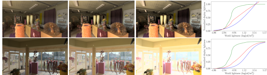
Fig. 7. Two opposite views in a same scene, a dark side (top) and a bright side (bottom). From left to right: the viewport TMO V(L_w(x, y), t) (blue curve), the combination of viewport and global TMOs L_d(G, V) (red curve), and the global TMO G(L_w(x, y)) (green curve).
