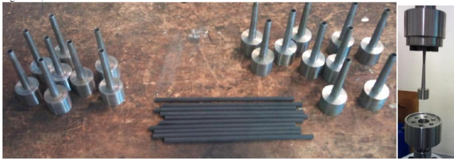
Figure 3. Carbon/epoxy rods, attaching parts, and testing systems
