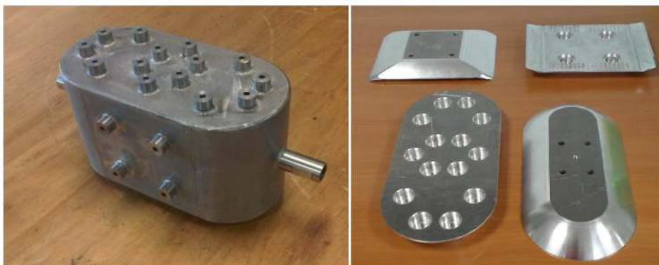
Figure 8. Form fitted liner made of stainless steel – aluminium shape adapter
