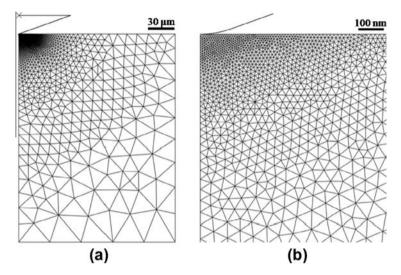
Fig. 6. (a) Overall mesh used for axisymmetric finite element modelling and (b) magnified view of the mesh close to the tip defect.
