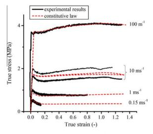
**Fig. 5.** Experimental stress–strain curve obtained from compression tests and corresponding deduced constitutive law.
