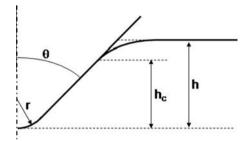
Fig. 2. Schematic representation in 2D of the nanoindentation test with a blunt equivalent cone.
