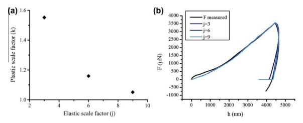
Fig. 9. (a) Series of pair solution identified defining the material properties and (b) loading and unloading cycle simulation for each pair solution (j, k).
