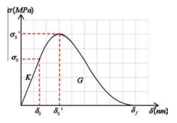
**Fig. 10.** Traction-separation behaviour with a failure mechanism used to account for the adhesive behaviour.
