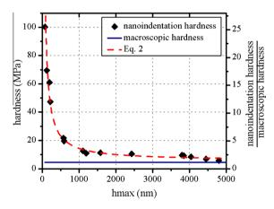
**Fig. 3.** Equivalent hardness  $H_u$  versus maximal indentation depth  $h_{\max}$  at  $\frac{h}{h} = 0.04 \text{ s}^{-1}$ .
