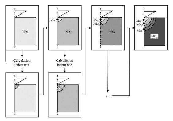
Fig. 7. Scheme of resolution for the calculation of the various zones used to account for the identation size effect.
