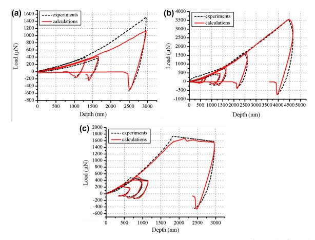
**Fig. 11.** Comparison between different experimental nanoindentation tests and corresponding numerical calculations: (a)  $\frac{h}{h} = 0.004 \text{ s}^{-1}$ , (b)  $\frac{h}{h} = 0.04 \text{ s}^{-1}$  and (c)  $\frac{h}{h} = 0.4 \text{ s}^{-1}$ .
