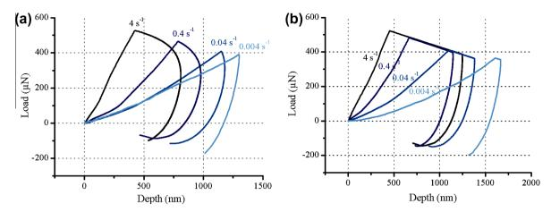
**Fig. 1.** Force–displacement curve of experimental nanoindentation tests at 4 different ratio  $\frac{h}{h}$ : (a) nanoindentation curves obtained without holding time between loading and unloading and (b) curves obtained with a holding time of 10 s.
