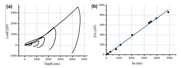
**Fig. 4.** (a) Nanoindentation curves obtained at  $\frac{h}{h} = 0.04 \text{ s}^{-1}$  showing the adhesion force  $F_a$  and (b) linear relationship between adhesive force  $F_a$  and the penetration depth  $h_a$  to loss of contact.
