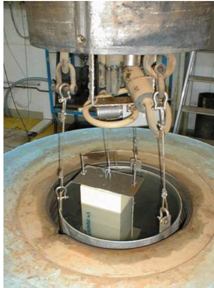
Figure 2 : Hydrostatic compression test
