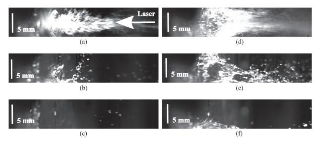
FIG. 5. Images extracted from the High-speed video (20 000 images/s) of water ejection for incident power densities of  $1 \text{ GW/cm}^2$  ((a)  $t = t_0$ , (b)  $t = t_0 + 2.2 \text{ ms}$ , and (c)  $t = t_0 + 5.5 \text{ ms}$ ) and  $3 \text{ GW/cm}^2$  ((d)  $t = t_0$ , (e)  $t = t_0 + 2.2 \text{ ms}$ , and (f)  $t = t_0 + 5.5 \text{ ms}$ ) and a spot diameter of 1 mm. The surface flow rate is 1 m/s.
