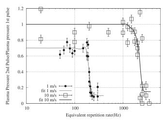
FIG. 9. Pressure rate between the peak pressure of the second pulse and the first one as a function of delay between two pulses (given at an equivalent repetition rate) for two surface flow rates of 1 and 10 m/s. The spot diameter is 1 mm, and the incident power density is 3 GW/cm<sup>2</sup>.
