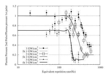
FIG. 8. Pressure ratio between the peak pressure of the second pulse and the first one as a function of delay between two pulses (given at an equivalent repetition rate) and incident power densities of 1, 2, and 3 GW/cm<sup>2</sup>. The spot diameter is 1 mm. The water flow is 1 m/s.
