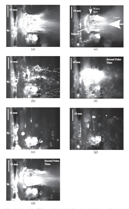
FIG. 4. Images extracted from the high-speed video (5000 images/s) of water ejection for two laser pulses in the water confinement regime at equivalent repetition rates of 50 Hz ((a)  $t = t_0$ , (b)  $t = t_0 + 5$  ms, (c)  $t = t_0 + 19$  ms, and (d)  $t = t_0 + 20$  ms) and 200 Hz ((e)  $t = t_0$ , (f)  $t = t_0 + 5$  ms, and (g)  $t = t_0 + 19$  ms). The incident power density is 3 GW/cm<sup>2</sup>, and the spot diameter is 3 mm. Surface flow rate: 1 m/s.
