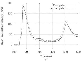
FIG. 7. Typical RFSV measurements by VISAR at 3 GW/cm<sup>2</sup>. The spot diameter is 1 mm, and the equivalent repetition rate is 50 Hz. (a) Without the cross-jet and (b) With the cross-jet.
