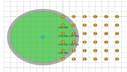
Fig.3 : Linear topology with 37 nodes
