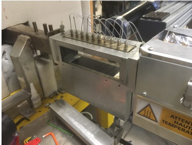
Figure 9. Pressure taps set up for B2A
