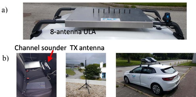
Fig. 4. a) Monopole antennas used in the setup, mounted on the aluminium sheet, on a vehicle roof, b) DoA measurement bench.
