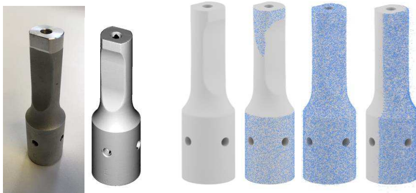
Figure 1: Real sonotrode (a1) scanned to get point clouds that have been post-treated (a2). CAD model of a sonotrode (b1) virtually reverse engineered following three parameterizations of the proposed framework (b2-b4).
