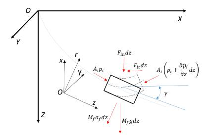
Figure 7: Forces acting on an internal fluid element
