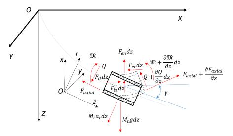
Figure 6: Forces and moments acting on an infinetesimal element of the drillstring
