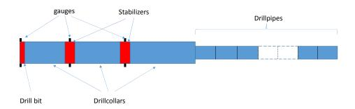
Figure 11: Drillstring assembly
