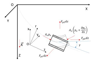
Figure 9: Sketch for calculating forces due to gravity and hydrostatic pressure
