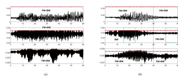
Figure 15: Radial displacement at the Nodes 10 (first row subfigures), 49 (second row subfigures, 282 (third row subfigures): without fluid (a), with fluid (b). The red dashed lines represent the drillstring-borehole clearances. The abscissa is the simulated time [s] while the coordinate is the displacement amplitude [m].
