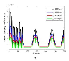
Figure 20: Viscous damping coefficient  $C_f$  under: (a) flow rate effect, (b) fluid density effect
