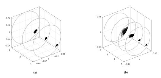
Figure 19: The Node 49 orbits under: (a) flow rate effect - (1)  $Q_f$ =0.01 m³/s, (2)  $Q_f$ =0.04 m³/s, (3)  $Q_f$ =0.06 m³/s; (b) fluid density effect - (1)  $\rho_f$ =1200 kg/m³, (2)  $\rho_f$ =1500 kg/m³, (3)  $\rho_f$ =1800 kg/m³, (4)  $\rho_f$ =2100 kg/m³
