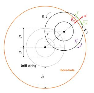
Figure 4: Drillstring borehole interaction
