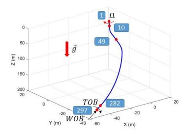
Figure 10: 3D well trajectory
