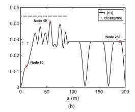
Figure 13: Quasi-static position of drillstring: (a) longitudinal and lateral displacements, (b) radial displacement
