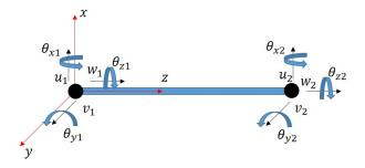
Figure 3: The 6 dofs per node of the beam element
