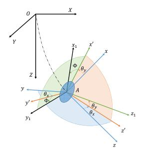
Figure 2: Transformation from undeformed to deformed states
