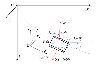
Figure 8: Forces due to annular flow
