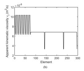
Figure 14: Drilling fluid parameters calculation at each finite element: (a) viscous damping coefficient  $C_f$ , (b) apparent kinematic viscosity  $v_f$
