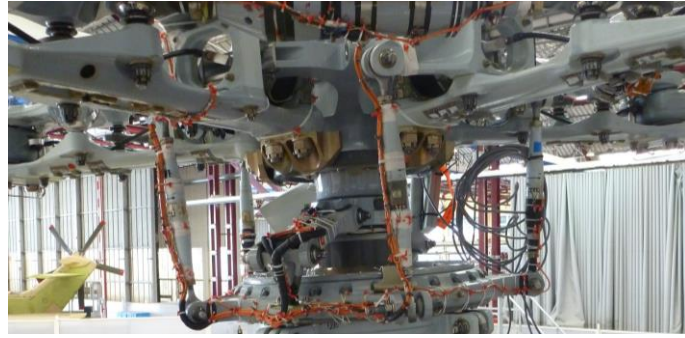
Figure 1. Instrumentation of a main rotor for flight testing
