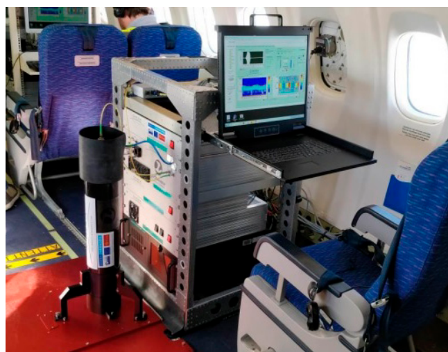
Figure 6. Picture of LIVE lidar installed inside the ATR42.
