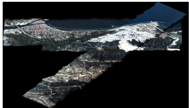
Figure 2: Mosaic of hyperspectral acquisitions above the refinery area using Hypspx hyperspectral instrument. The refinery appears as the bright part near the coastal area (Berre Pound).
