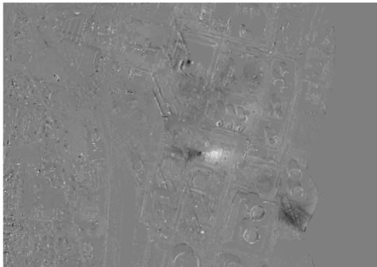
Figure 13 : Extract of the 10am differential image (first change of wind direction in the morning) in mass (g) above CH11 boiler (scale range [-0.05: 0.05]).
