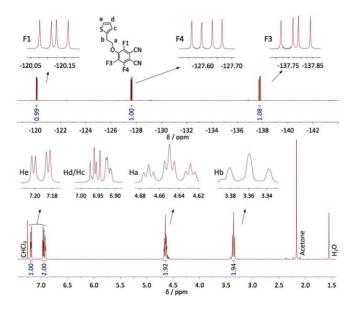
**Fig. 1** <sup>1</sup>H (bottom) and <sup>19</sup>F NMR (top) spectra of **1a** in CDCl<sub>3</sub>, with the integration values; the identification of all H and F atoms is given.
