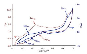
**Fig. 3** CV of **5**, on Pt disc electrode, in DMF containing 0.1 M  $Bu_4NPF_6$ , at a scan rate of 0.1 V  $s^{-1}$ , at a concentration of  $10^{-3}$  mol  $L^{-1}$  (solid blue line) and at  $4x10^{-3}$  mol  $L^{-1}$  (aggregation, dashed red line).
