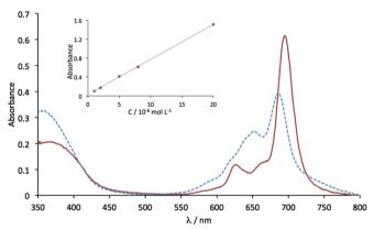
**Fig. 4** UV-visible absorption spectra of **5** in chloronaphthalene (solid red line) and in dimethylformamide (dotted blue line), both at 8x10<sup>-6</sup> mol L<sup>-1</sup>. The inset shows the variation of the absorbance at the maximum wavelength as a function of the concentration, in chloronaphthalene.
