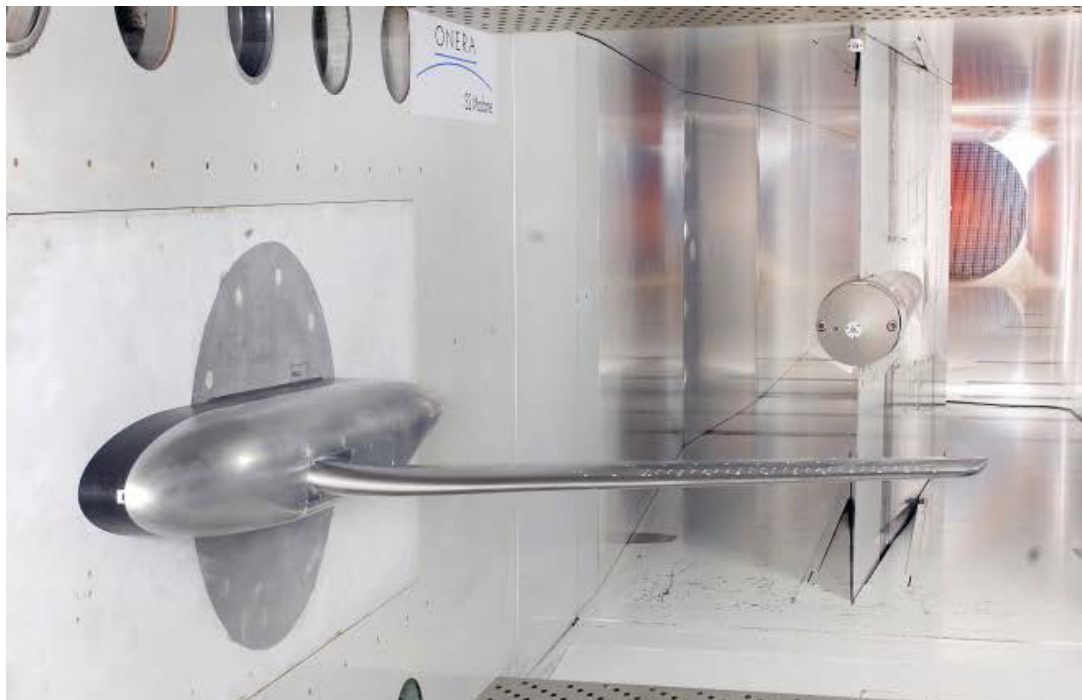
Figure 8: 3D model in the ONERA S2MA wind tunnel.
