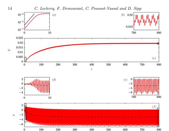
FIGURE 5. Timeseries of (a, b, c) perturbation kinetic energy E and (d, e, f) shear-stress measurement y of the unforced flow, with sliding mean shown as a black dotted line. Zooms on the initial and final stages are shown in insets.
