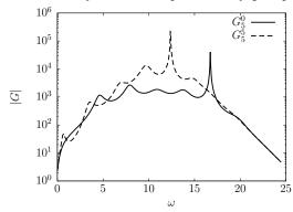
FIGURE 18. Comparison between the gain of the transfer functions  $G_5^0 = G_b$  associated with the base flow only and  $G_5^5$ , the transfer function associated with the closed-loop between the base flow and the final controller  $K_5$ .
