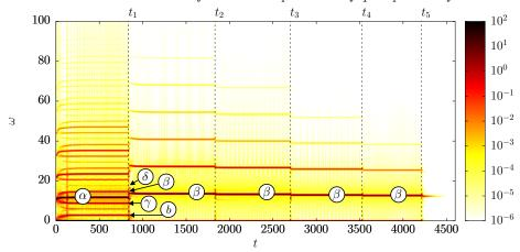
FIGURE 8. Spectrogram of the timeseries y(t), using short-time Fourier analysis with Hamming windows of length T=20 and 50% overlap. In this section, we focus on the unforced flow for  $t< t_1$ , but further comments regarding the controlled flow are provided in §5.2. Resonant mean-flow modes  $\alpha, \beta, \gamma, \delta$  and b are indicated, according to modal analysis reported in §3.5 and §5.3. The start-up time  $t_m$  of each controller correction  $K_m'$  is shown with a dashed line.
