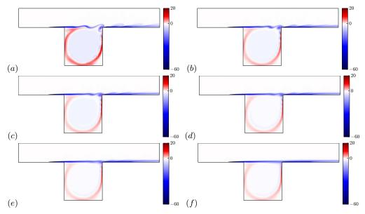
FIGURE 15. Vorticity snapshots at a time where the shear-stress measurement y is maximum (a) m = 0, (b) m = 1, (c) m = 2, (d) m = 3, (e) m = 4, (f) m = 5. The colormap has been cropped to the same arbitrary extremal values in all plots for comparison.
