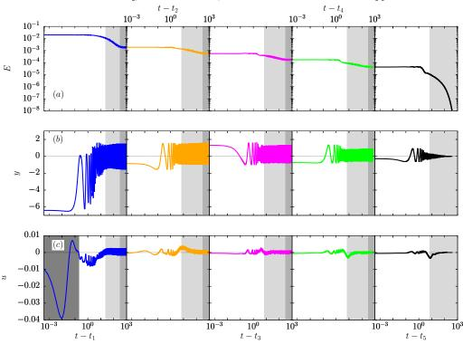
FIGURE 13. Timeseries of (a) the perturbation kinetic energy E, the sensor perturbation y and the control signal  $u = \sum_m u_m'$  for the controlled flow. The time axis is in log scale to highlight the different time-scales. For each iteration m, the time origin is reset to zero by subtracting  $t_m$ , the start-up time of the new controller  $K_m'$ , so that the first point is at  $\mathrm{d}t = 4 \times 10^{-4}$  in each panel.
