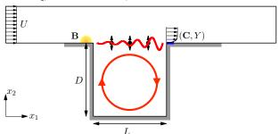
FIGURE 1. Numerical model of open cavity flow, with upstream (volume force) actuator B (in vellow) and downstream (shear-stress) sensor  $(\mathbf{C}, Y)$  (in blue). The shear-layer instability and cavity recirculation are symbolized with red lines. There are three  $x_2$ -velocity probes in the shear layer at  $x_2 = 0$  and respectively  $x_1 = 1/4, 1/2, 3/4$ . Grey thick lines indicate no-slip boundary conditions.
