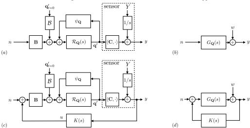
FIGURE 3. Block diagram of the forced Navier–Stokes equations in the (a) open-loop case and the (c) closed-loop case. Equivalent representation with an open-loop transfer function  $G_{\mathbf{Q}}$  from n to y and an output disturbance w in (b) the open-loop and (d) the closed-loop.
