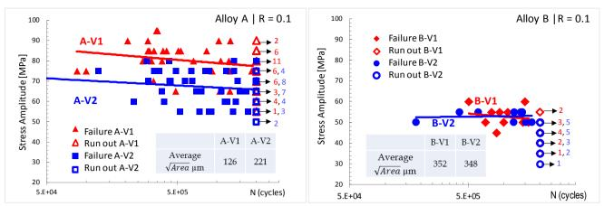
Figure 11: SN-Curves plotted in semi-Linear diagram for the batches A-V1, A-V2, B-V1 and B-V2
