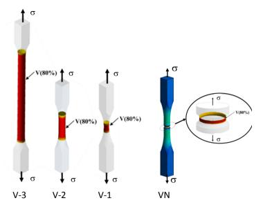
Figure 10: Highly Stressed Volume for (a) smooth specimens V1, V2 and V3 and (b) notched specimens
