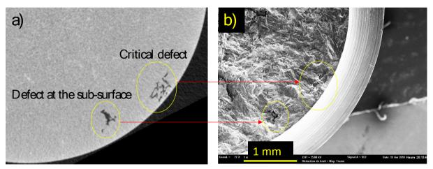
Figure 31: specimen B-VN-05 (a) tomographic image and (b) its corresponding fractographic image
