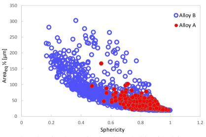
Figure 4: Defect size as a function of the sphericity of the defects
