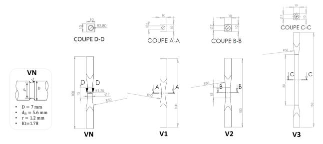
Figure 5: Specimens for tensile fatigue tests
