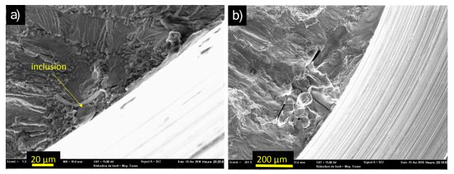
Figure 30: Fatigue failure, (a) specimen A-VN-05, Sa=70 MPa, Nf=1584002 cycles, crack initiation from an inclusion with  $\sqrt{Area}$  of 27 µm (b) specimen B-VN-05, Sa=45 MPa, Nf=777402 cycles and crack initiation from a pore at the surface with  $\sqrt{Area}$  of 313 µm
