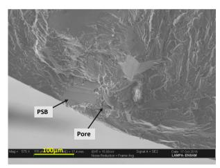
Figure 17: The presence of some sites with the combination of two mechanisms, crack initiation from persistent slip band (PSB) and pore near to the surface
