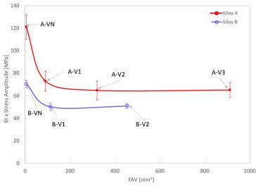
Figure 12: Local stress amplitude at fatigue limit as function of critical volume for alloys A and B
