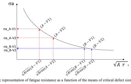
Figure 26: Schematic representation of fatigue resistance as a function of the means of critical defect size for each batch
