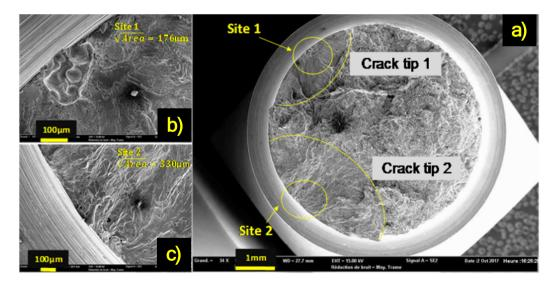
Figure 15: Specimen with multiple crack initiation sites, specimen B-NV-04, Sa=45MPa, Nf=129663 cycles, crack initiation from a pore at surface (a) Macroscopic view, detailed view of (b) gas pore and (c) micro-shrinkage pore
