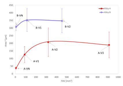
Figure 19: The critical defect size as a function of the Fatigue Active Volume
