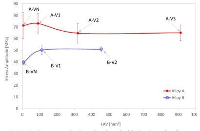
Figure 13: Nominal stress amplitude as function of critical volume for alloys A and B
