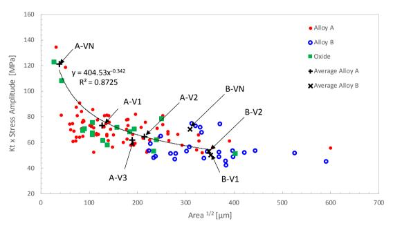
Figure 25: Local fatigue resistance as a function of critical defect size (R=0.1)
