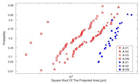
Figure 22: Critical defect sizes in √area plotted on lognormal probability papers
