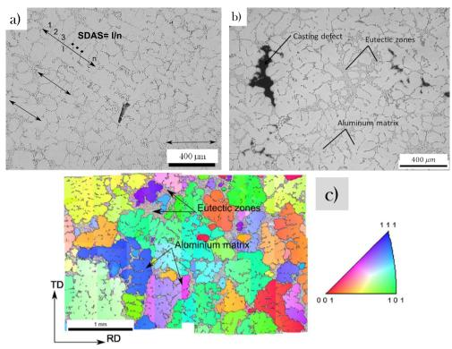
Figure 1: The microstructure of the investigated alloys (a) Alloy A (AlSi7Cu05Mg03 - T7) (b) Alloy B (AlSi7Mg03 - T7) and (c) Grain map showing grains for alloy A with  $\sqrt{Area \, (grain)} = 337 \pm 143 \, \mu m$ .
