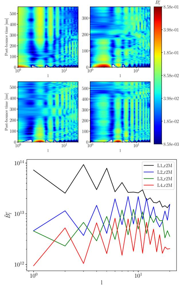
**Figure 15.** Harmonic decomposition of the radial component of the magnetic field at the PNS surface for models  $L^*_r2M$  as defined in equation (18) (top panel) and spectra taken at  $t = 358$  ms p.b. (bottom panel).
