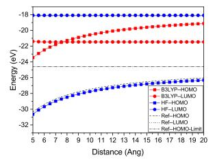
FIG. 3. HOMO and LUMO orbital energies as a function of the donor-acceptor distance for the N-2 Be $\cdots$ He system. HF predicts the energies well with the correct HOMO-LUMO energy ordering in both short and long distances. However, B3LYP predicts an unphysical energy crossing at around 7.5 Å and therefore gives non-Aufbau results after the crossing.
