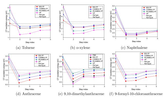
FIG. 7. Stepwise analysis on the pp-RPA calculation for molecules within benzene, naphthalene, and anthracene families.
