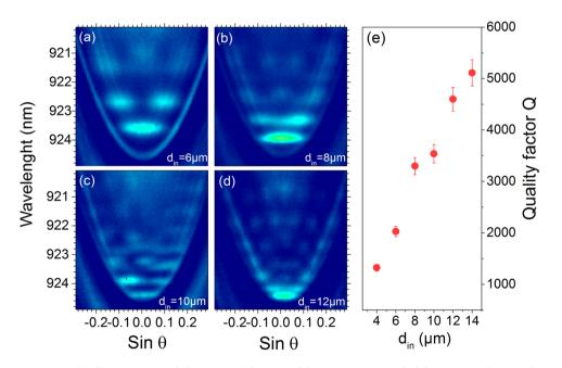
**Figure 5.** (**a**–**d**) Experimental dispersion relations of the emission recorded for rings with inner diameter  $d_{in}$  of 6, 8, 10, and 12 µm. (**e**) Variation of the confined super Tamm fundamental mode quality factor as a function of  $d_{in}$ .
