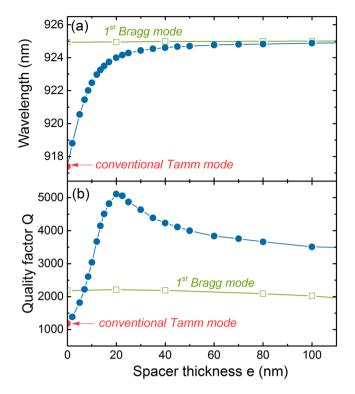
**Figure 2.** Variation of (a) resonance wavelength and (b) quality factor with the spacer thickness calculated by the transfer matrix method. The spacer (n = 1.485) is either inserted between a 65 pairs DBR and a 45 nm thick silver layer (blue circles) or deposited on a 65 pairs DBR without metal (green open squares).
