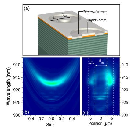
**Figure 4.** (a) Schematic representation of the sample evidencing the DBR, the PMMA resist layer (e = 35 nm) and the 45 nm silver layer. Rings of inner diameter  $d_{in}$  and arm width L are defined in the PMMA layer. (b) Experimental emission dispersion relation recorded on a ring of inner diameter  $d_{in} = 6 \mu m$ . (c) Wavelength-resolved emission as a function of the position along the diameter of the ring.
