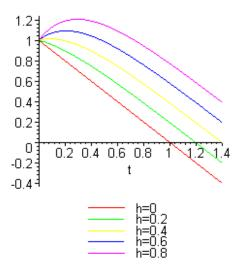
Figure 2.  $(D/D_i)^2$  as a function of reduced time  $\tau = K_{os} t/D_i$ , for  $\tau_T = 0.3$ , for a subcritical droplet.
