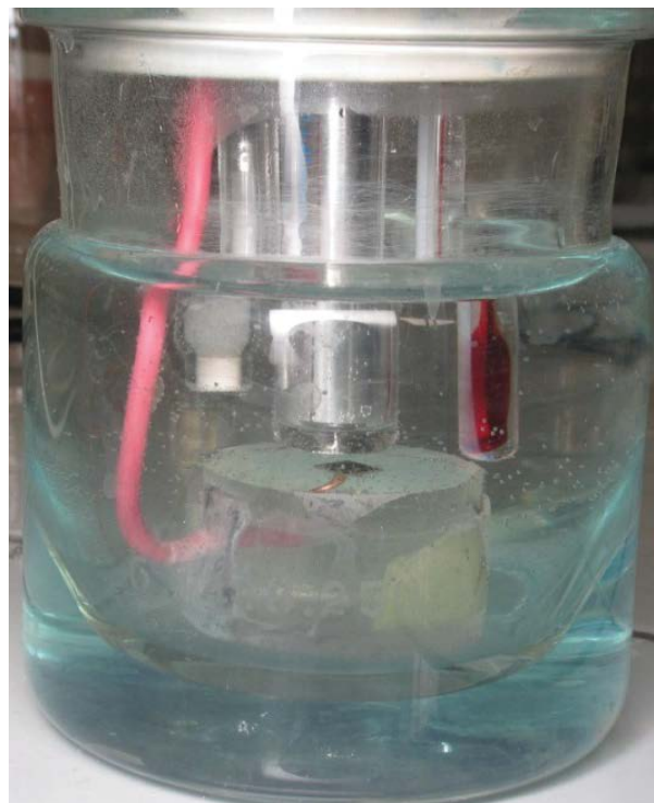
Figure 2 Photograph of the double-envelope cell with the three positioned electrodes.
