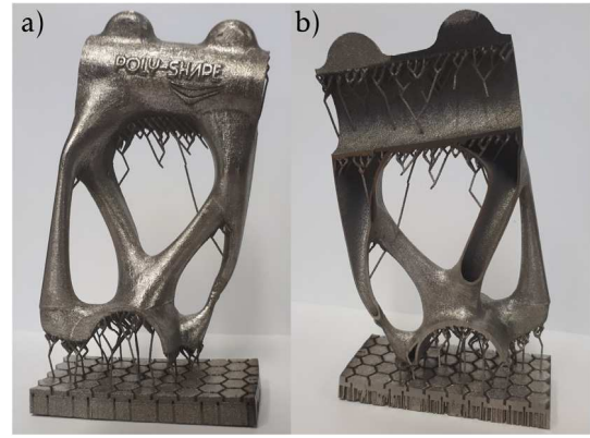
Fig. 18. The Stem test case printed in LBM and sawn in two to make internal supports visible.
