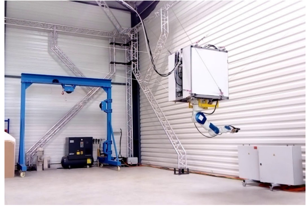
Fig. 1. Cable-driven parallel robot CoGiRo with a 7-DOF robotic arm.
