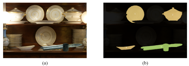
Figure 10: (a) Spliced image, (b) Estimation of the illuminant color in the RGB color space, with enhanced saturation.
