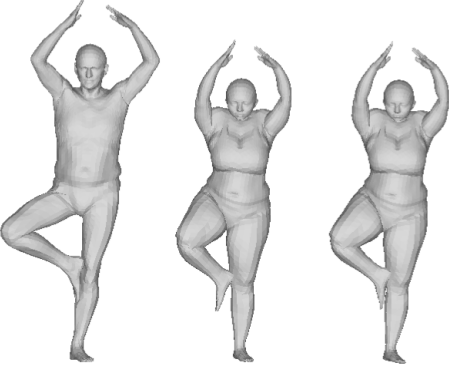
(b) Left to right: source pose, transfer result without attraction term, and with attraction term (target from Figure 6b). The right foot does not penetrate the leg thanks to the repulsion term, but needs the attraction term to keep the contact present in the source pose.
