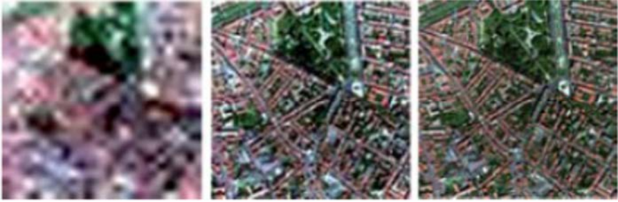
Figure 1.5. Images of Toulouse at three spatial resolutions of 30, 8 and 2 m generated from data obtained from the airborne multispectral camera PELICAN during the Musarde experiment (ONERA/IGN credit, 2010). For a color version of this figure, see www.iste.co.uk/baghdadi/5.zip
