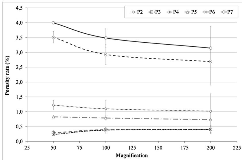
Fig. 12. Porosity rate of 5 samples according to the micrographic magnification (analyzed surface = 19 mm<sup>2</sup>).
