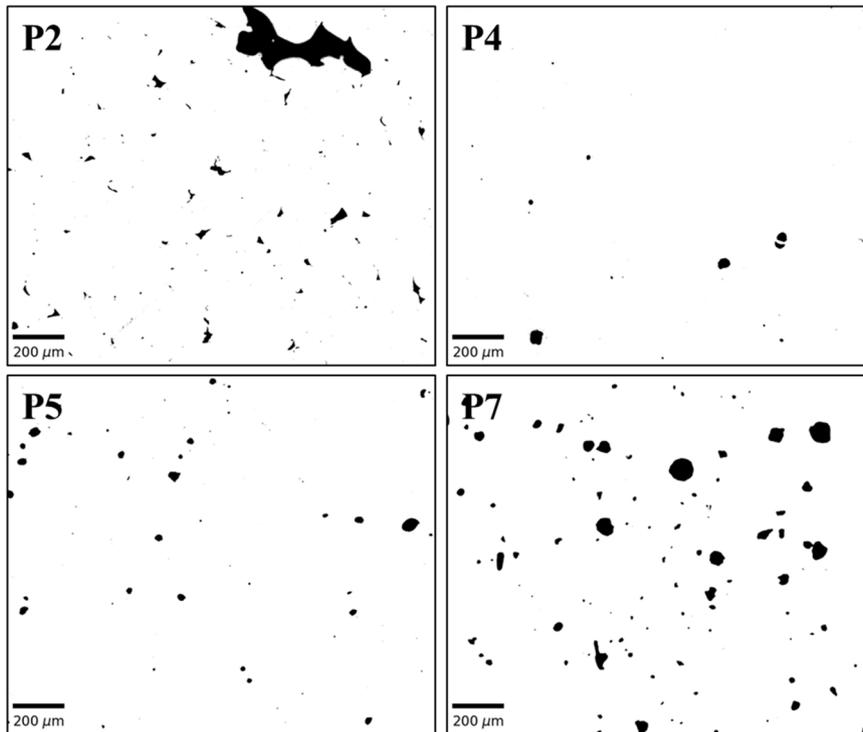
Fig. 16. Micrographic cross-sections of samples P2, P4, P5 and P7 samples (50, 100, 125 and 250 J/mm<sup>3</sup>) corresponding to respectively 1.8%, 1.1%, 1.7% and 5% porosity rates (Archimedes method).
