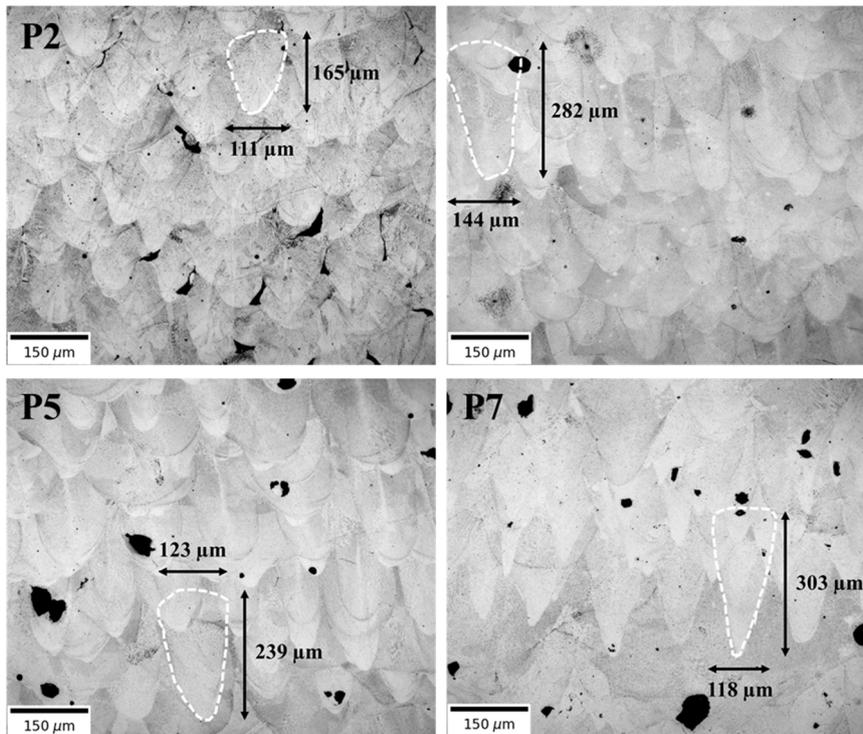
Fig. 17. SLM microstructures after chemical etching. Analysis of bead dimensions for samples P2, P4, P5 and P7 samples (50, 100, 125 and 250 J/mm<sup>3</sup>).
