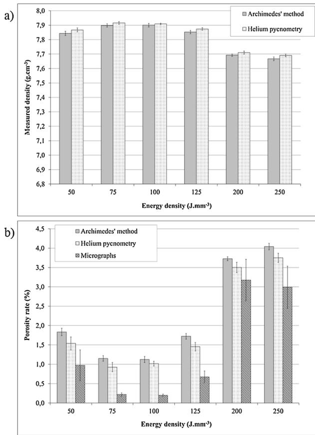
Fig. 14. (a) density measurements and (b) porosity rate estimation for P2 to P7 samples (50–250 J/mm<sup>3</sup>).
