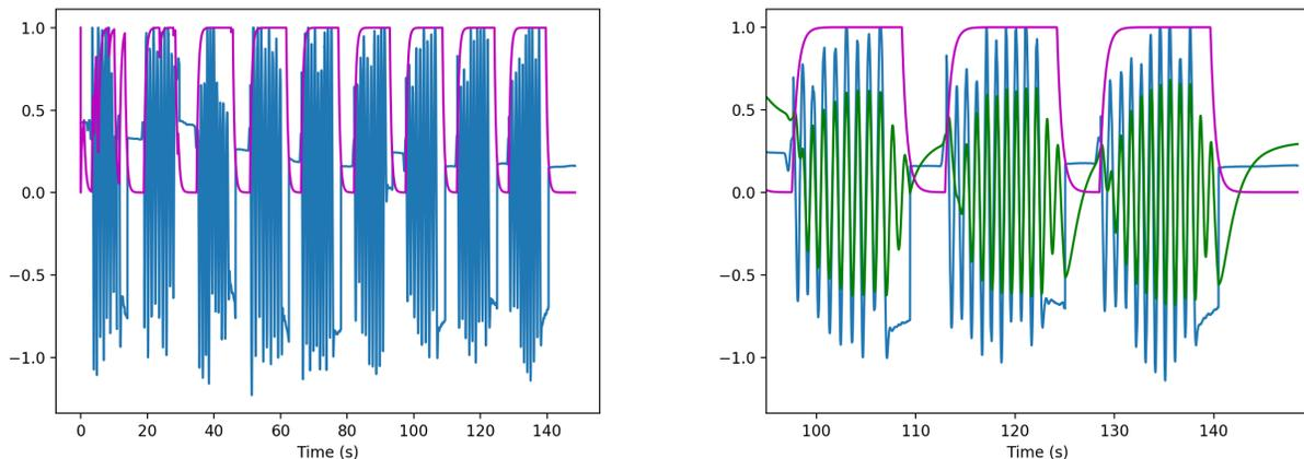
Figure 4: Left: Example of classification result. In blue, the CPG input, in magenta, the evolution of  $\sigma_f$ , i.e. classification result (1 for rhythmic and 0 for discrete). Right: Zoom over the results. In blue, the CPG input, in green the CPG output, in magenta, the evolution of  $\sigma_f$
