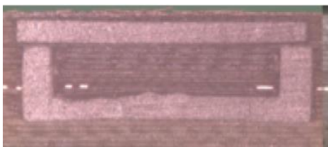
Figure 16: Cross section of the embedded flyback transformer, showing the magnetic core and the copper windings.
