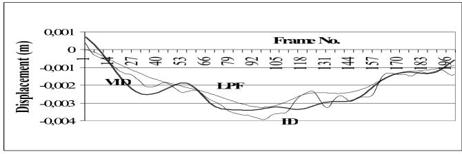
Fig. 2. Antero-postérior excursions of the center of mass calculated by the video (VID), low-pass filter (LPF) and inverse dynamic (ID) methods.
