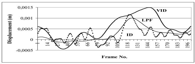
Fig. 3. Medio-lateral excursions of the COM calculated by the video (VID), low-pass filter (LPF) and inverse dynamic (ID) methods.
