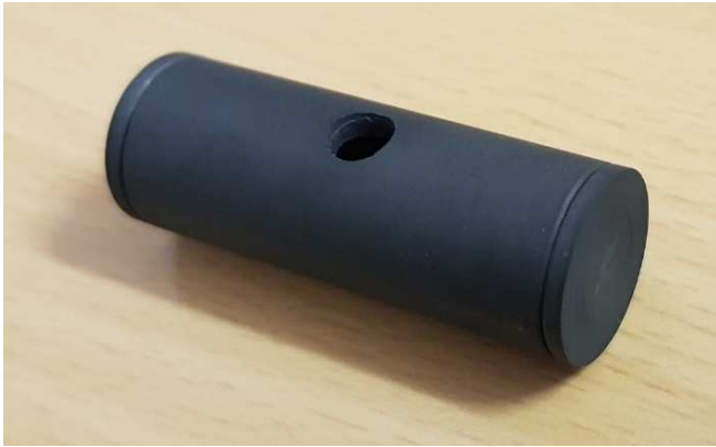
Fig. 2. Graphite holder used for the ^{169}\text{Er} separation. The erbium solution has been poured inside and evaporated to have a deposit on the graphite.
