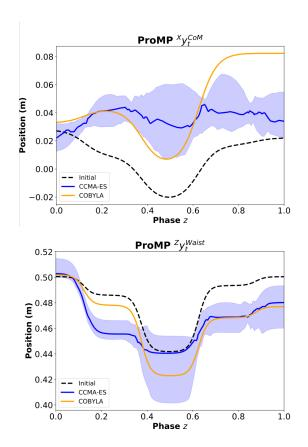
Fig. 8: Reference trajectories: initial (from human demonstrations) and after optimization. Both CCMA-ES and COBYLA were bootstrapped from a ProMP that combined every demonstration, *all*. The 30 reference trajectories for CCMA-ES are represented with their median and IQR.
