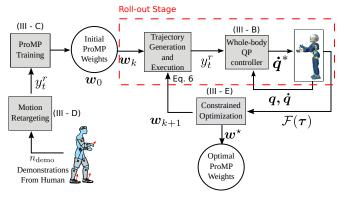
Fig. 2: Overview of our framework for learning optimal weight parameters for whole-body trajectories.
