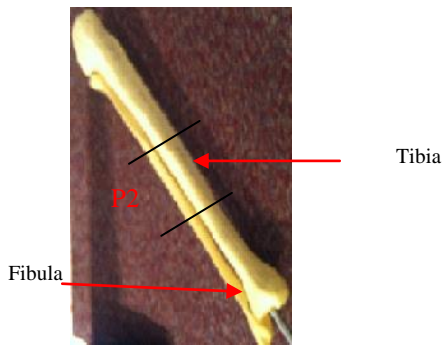
Fig.5. Sawbones™ composite bone mimicking phantom
