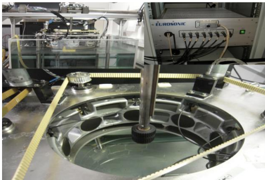
Fig.1. Ultrasonic Computed Tomography device (Copyright / Rights reserved, CNRS-LMA Marseille)[1]
