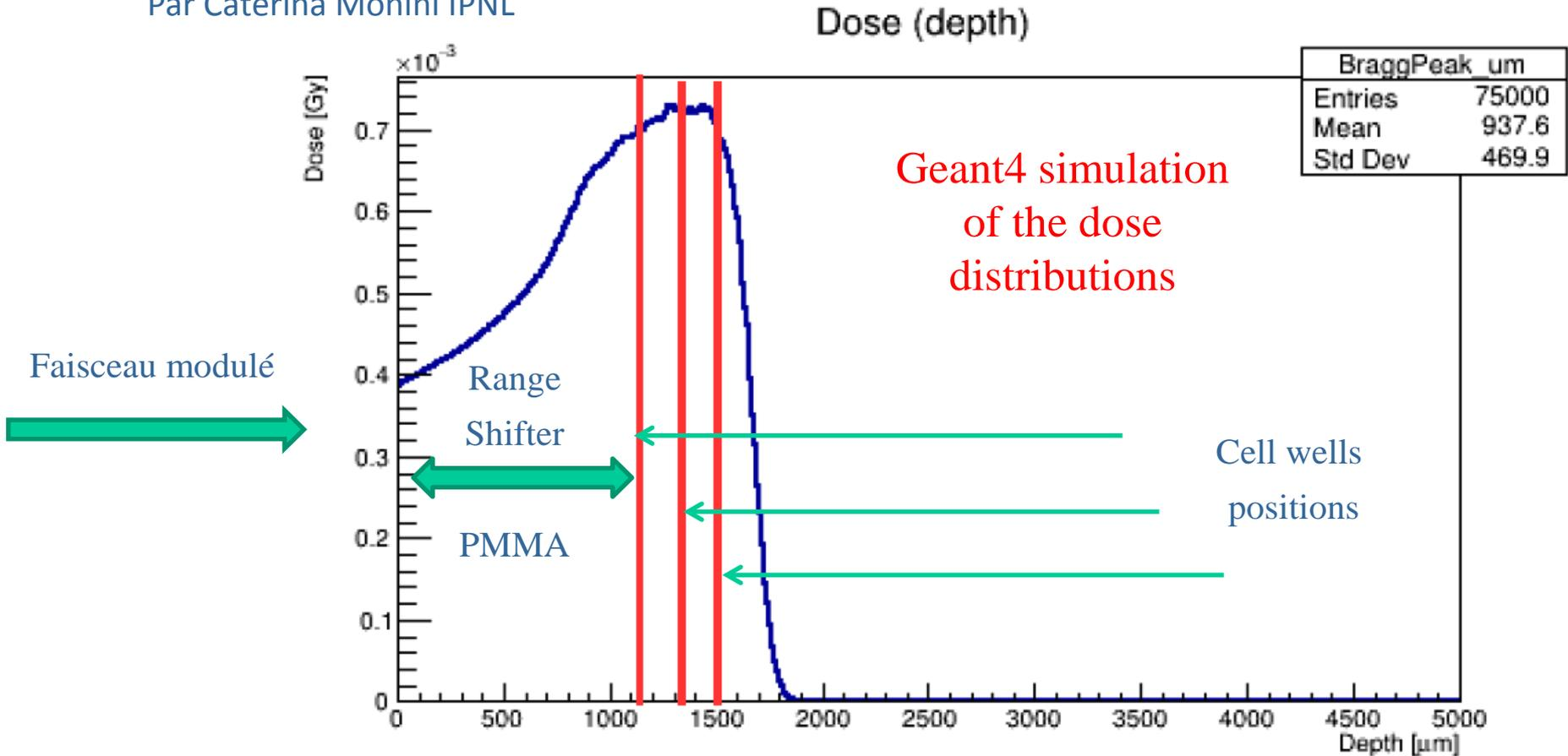
The dose homogeneity, in the SOBP region, was verified experimentally with the irradiation of radiochromic film stack
