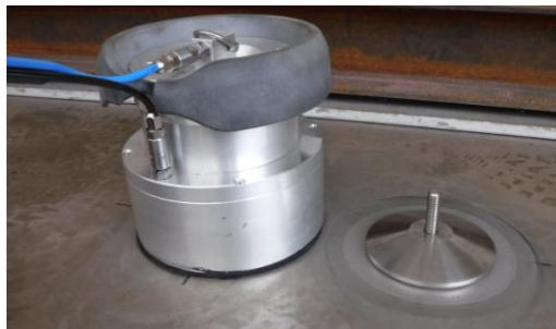
Fig. 1: Photo of the solution developed by Cold Pad (application disposal on the left and adhesively bonded fastener on the right)
