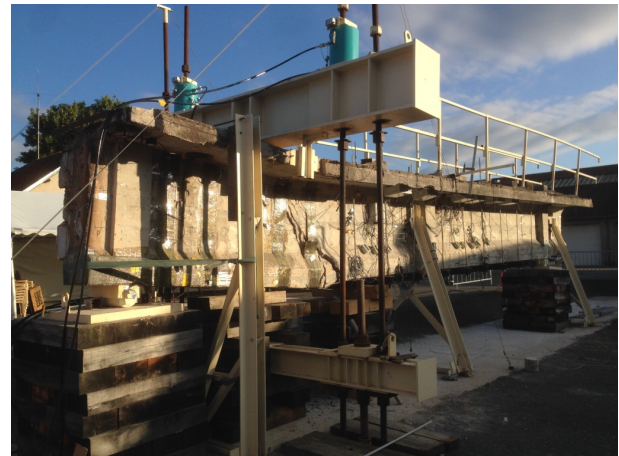
Fig. 12. Photo of the beam after the shear test up to failure
