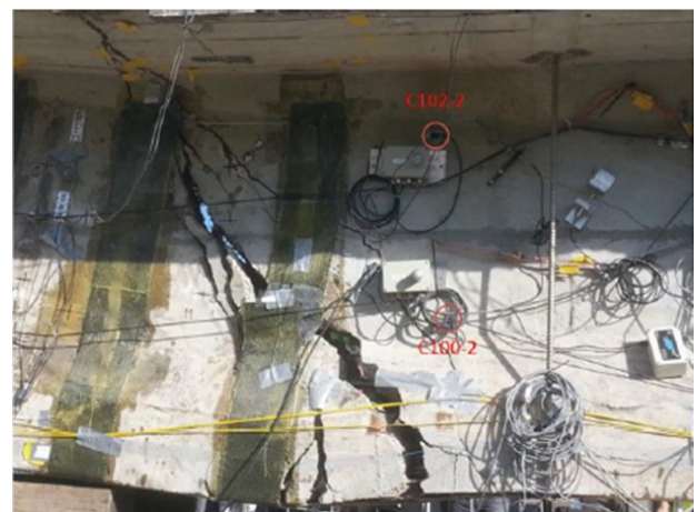
Fig. 13. Photo of the tested beam at the end of the shear test – detail of the main crack
