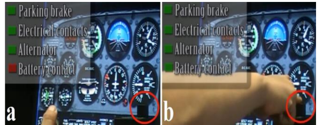
Figure 8: System management context. The system knows that the pilot must activate the battery contact. Therefore, a Tacsels containing a switch button (highlighted with a red circle) emerges near the pilot (a). The pilot notice the Tacsels and immediately press the switch button (b).
