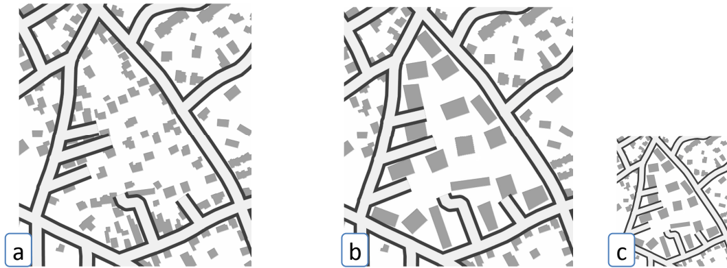
Figure 9. Instance of displacement of dead-end streets for a 1:50k map. (a) the original data (1:25k). (b) the generalized data for a 1:50k map. (c) same as (b) displayed smaller.
