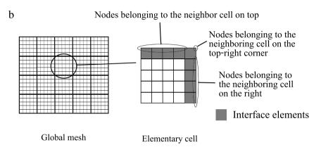
Fig. 2. Examples of 2D meshes and decomposition in elementary parts.
