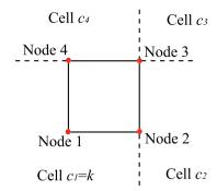
Fig. 3. Corner element: nodes and neighboring cells definition.
