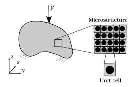
Fig. 4. Example of composite structure with periodic geometry.
