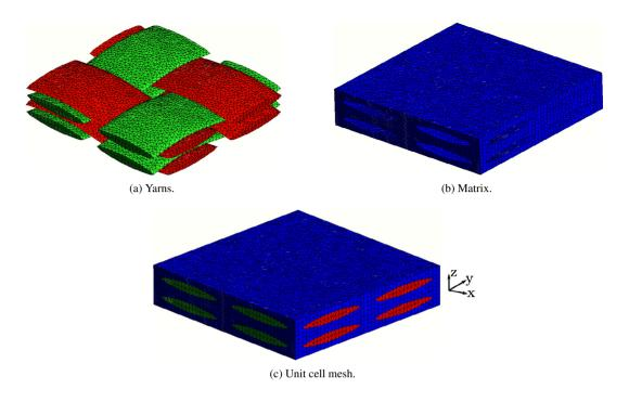
Fig. 11. Periodic tetrahedral mesh of unit cell model.
