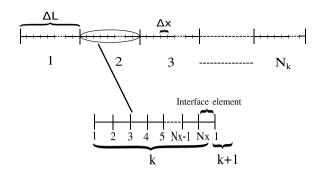
Fig. 1. 1D mesh and decomposition in elementary parts.
